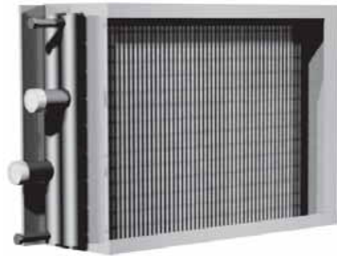
The QLTN casing with inward folded edges on the top and bottom plates as well as cover plates for the header and elbows.
