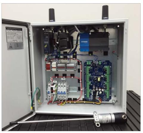
Shown is a typical data acquisition and control panel with a power meter and flow sensor.
