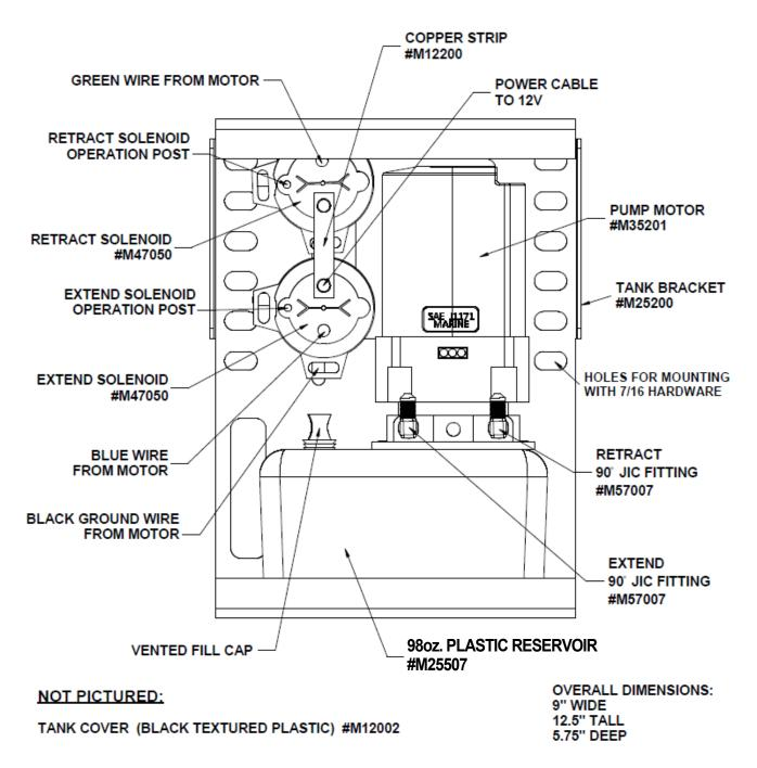
Replacement Assembly Standard motor: #M26850 Replacement Assembly Manual Override motor: #M26855
