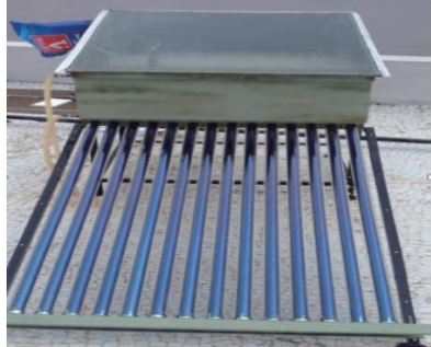
Fig.1 Experimental set up of double basin solar still with evacuated tubes
