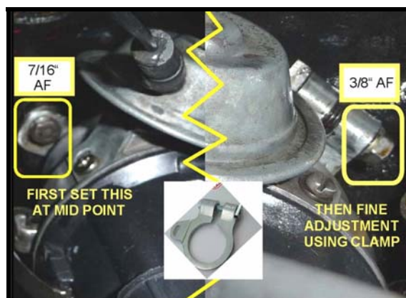
Figure 14 Distributor adjustment
