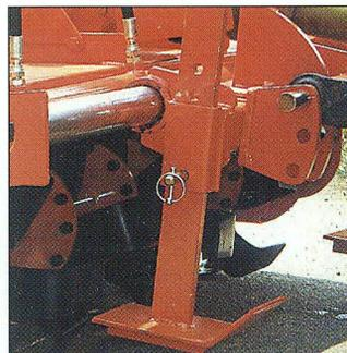
The front skids allows offset during working without side draft.
