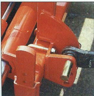
Detail of the lower link with three positions.
