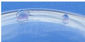
Fig 10. **Brinell HD** top coat contact angle after stroke test
