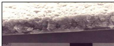
Fig 2. Standard thin film coating
