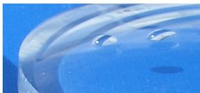
Fig 9. Standard top coat contact angle after stroke test
