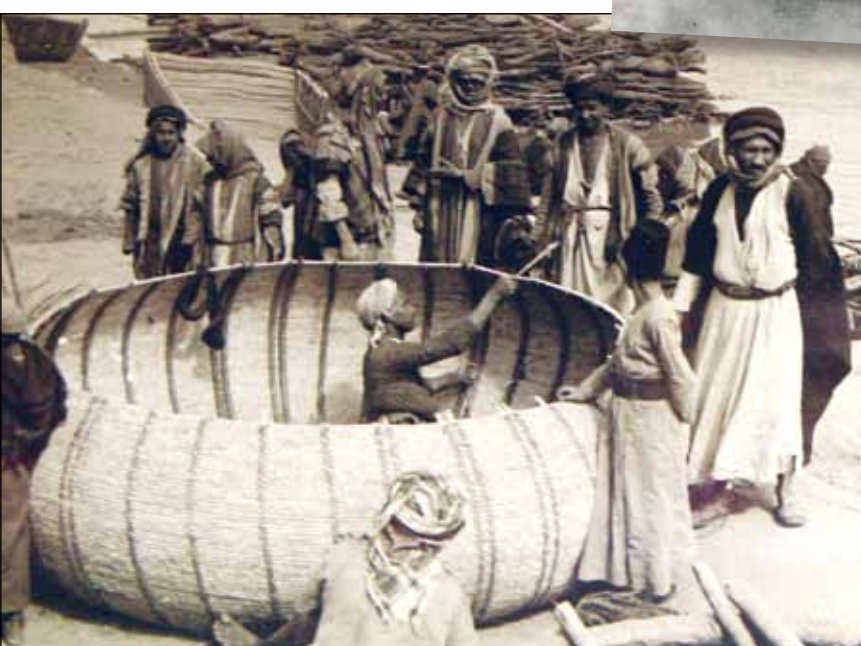
ABOVE Iraqi Marsh Arabs build a reed coracle. INSET Its design allows a coracle to be packed with cargo without compromising stability.
