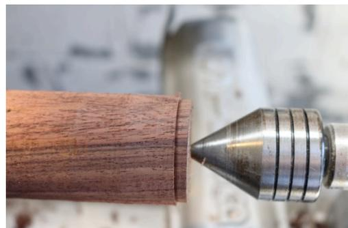
depth of the hole using the Forstner bit as a ruler then add  $\frac{1}{4}$ " and mark the top of the shaker. Turn 3 "V" cuts inside the 1" hole then sand the inside of the hole to remove burs. Remove the wood from the chuck and replace with the pipe nipple re-chuck.
