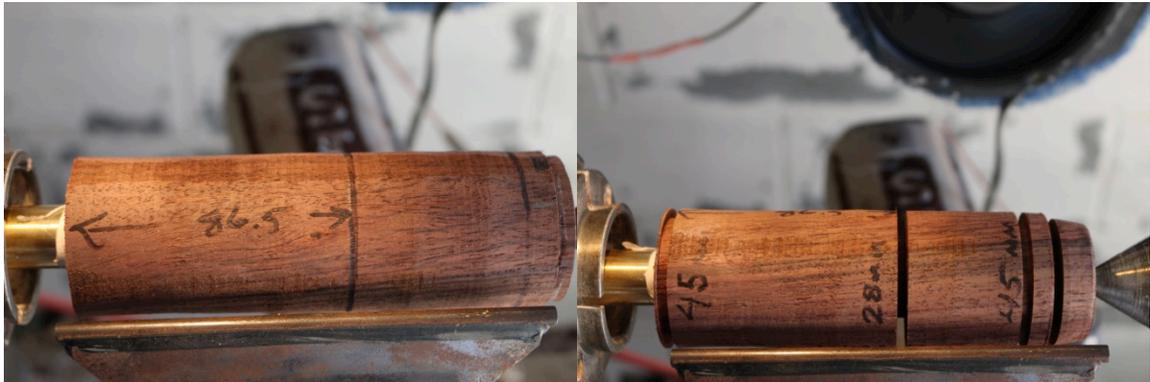
Max diameter is 46 mm and it is about 10 mm up from the bottom so the minimum diameter is:  $46/1.618 = 28.5$  mm which is at 86.5 mm. The wide area at the top is also about 10 mm down from the top.
