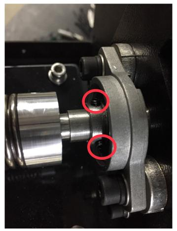
LOOSEN 2 SCREWS OF THE BACK BEARING, AND KNOCK THE FRONT END OF DRUM CHART(NO NEED TO LOOSE THE SCREW), MAKE SURE THE GAP ABOUT 2MM, THEN LOCK TWO SCREWS OF BACK BEARING AND TEST THE MACHINE.
