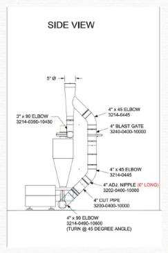
THIS IS JUST AN EXAMPLE OF AN APPROVED METHOD TO EXHAUST BOTH THE CHAFF UNIT AND COOLING TRAY FAN OUT OF BUILDING IF COMBINING THE TWO PIPES INTO ONE USING A BACKDRAFT OR BLAST DAMPER.
