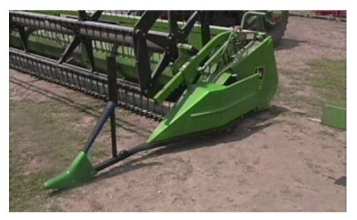
When you remove the old style dividers, removal of linkage mounted to reel lift arm is also required. The old springs will be replaced by new springs and adjustment bolts & nuts (included).
