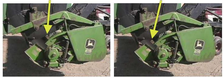
The bracket that the old spring is hooked into (above sickle drive) is mounted with 3 carriage bolts. Remove all 3 bolts, shift the spring bracket forward one set of holes, and remount with 2 bolts.
