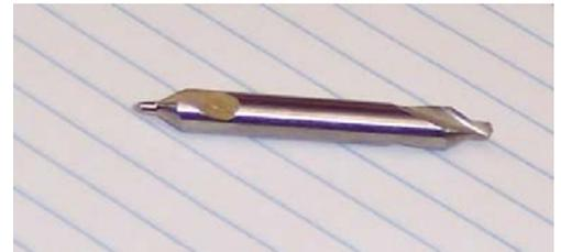
centerpoint used in preparation for drilling
