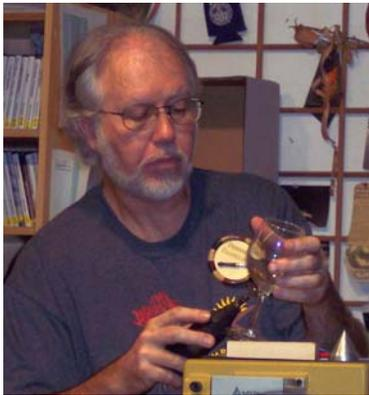
Using a Dremmel tool with a cut off blade, he cut off the stem by scoring a line around it just below the goblet part.
