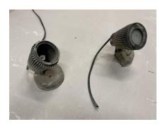
protect against corrosion. Powder coating is one common method.
