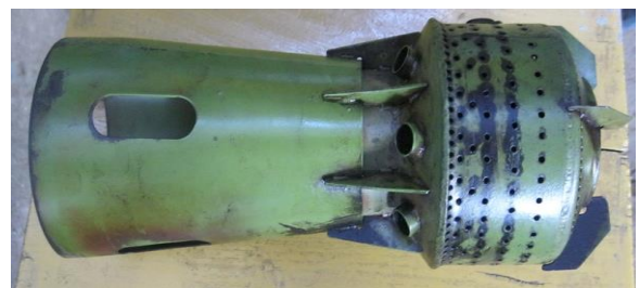
Figure 3: Tubular Combustor of Rover turbine
