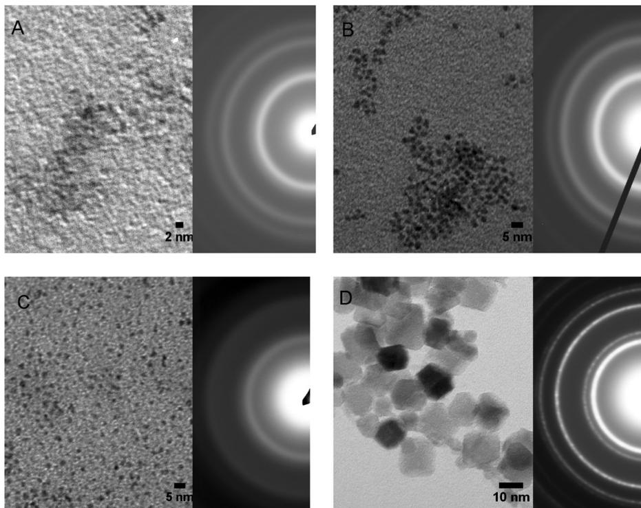
**Figure 2.** TEM images and electron diffraction patterns for four nanoparticle preparations: (A) 1.1 nm diameter, (B) 2 nm diameter, (C) 2 nm diameter (showing reproducibility), and (D) 11.8 nm diameter.
