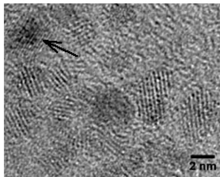
**Figure 1.** HRTEM image of 2 nm CeO<sub>2</sub> nanoparticles. The arrow indicates a difference from the rest of the nanoparticles (see text).
