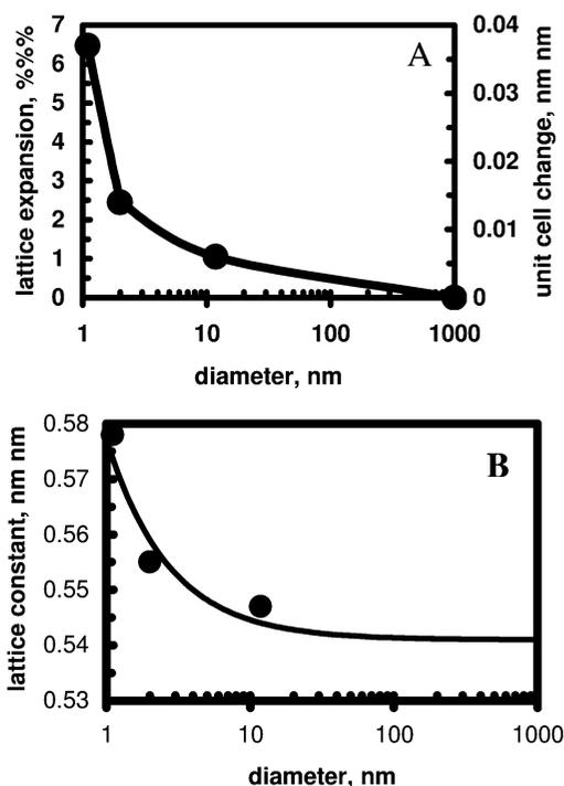
**Figure 3.** (A) Lattice constant vs particle mean diameter. The curve is defined by the equation given in the text. (B) Lattice expansion vs particle mean diameter.
