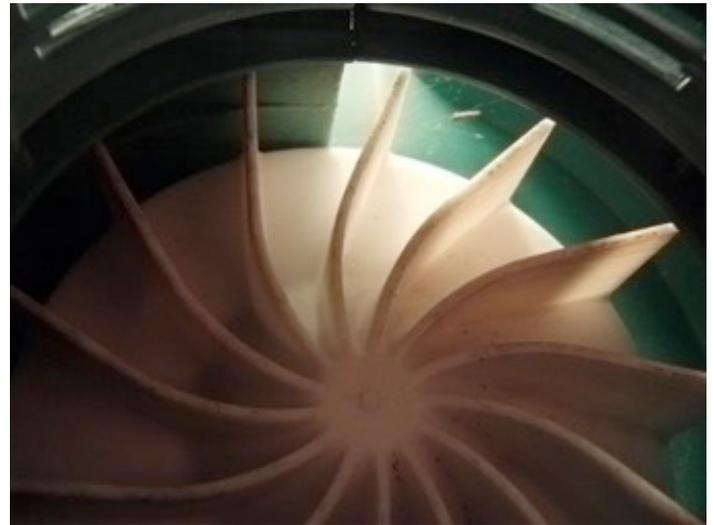
*Electric leaf blower vanes showing sharp edge in air escape vent*
