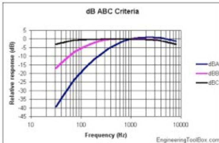
dB-A curve showing low frequency rolloff
