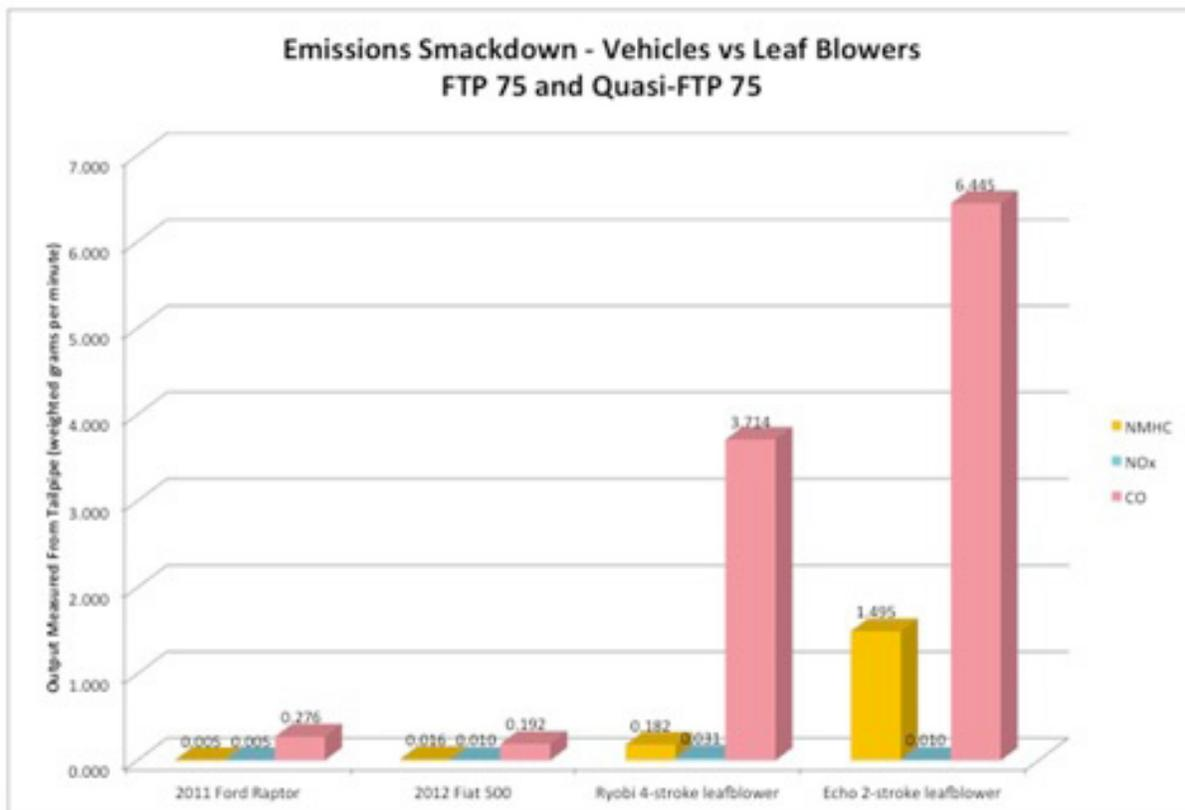
*Typical-use emissions of hydrocarbons, nitrous oxides and carbon monoxide.*
