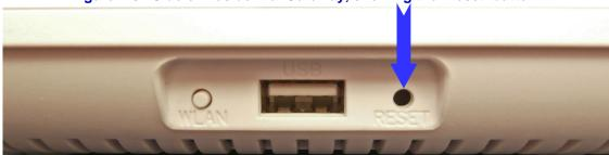
Figure 7-5. Side of Residential Gateway, showing the 'Reset' button.
