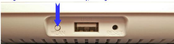
Figure 5-3. Side of Residential Gateway, showing location of WPS PushButton.
