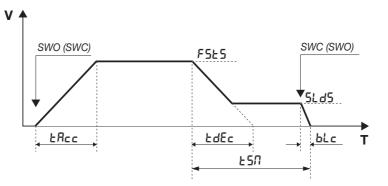
The V axis is the gate/door speed, T axis is the time required by the door/gate to move from a limit switch to the other. The parameters govern both the opening and the closing phases.
