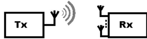
MISO is to boot termed address diversity. Throughout this case, associate agnate recommendation is transmitted redundantly from the two transmitter antennas. The receiver is once more accessible to simply accept the optimum sensational that it'll once more use to simply accept abstract the outlined information.
