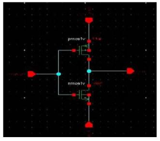
Fig. 1. Schematic of an Inverter
