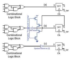
Fig. 3. Block diagrams of (a) original nonequalized design, (b) equalized design with onefeedback path ON, (c) buffer-inserted nonequalized design
