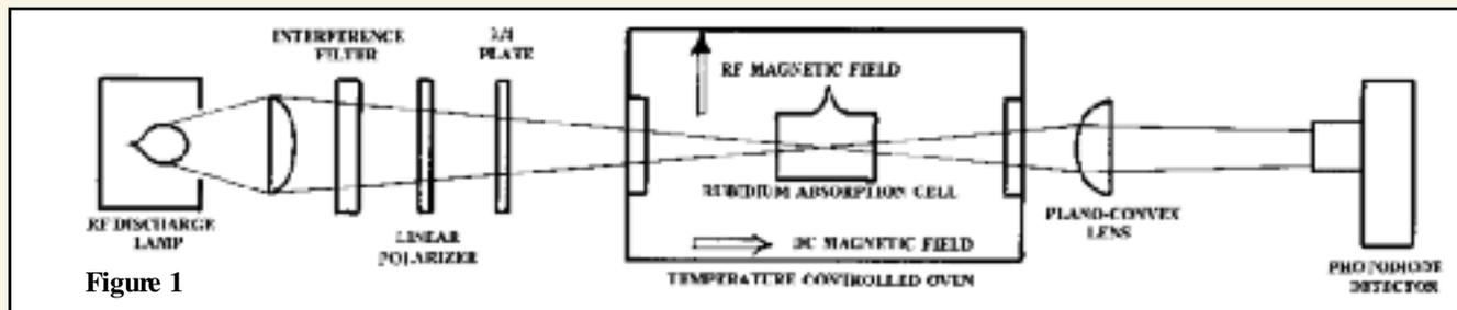
**Optical Pumping** is a widely used and powerful technique for exploring atomic energy states, atomic transitions, and atomic collisions using electromagnetism in the form of light, radio frequency, and uniform constant magnetic fields. TeachSpin's OP1-A explores the atomic physics of both isotopes of natural rubidium.
