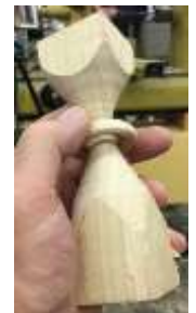
Set up for turning a captive ring. Left picture is set up for turning a captive ring and end picture is a turned captive ring
