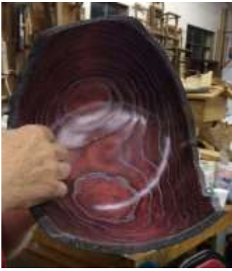
Ken Lindgren holds a natural edge bowl turned from Red Oak. He removed the center and then burned and wire brushed the outside. He used two colors of dye and liming wax inside. He first dyed the inside black, then sanded it off, except for what was in the pores of the wood. He then added red dye, two coats of finish and the liming wax. He plans carve a ring around the top rim and fill it with coffee grounds.
