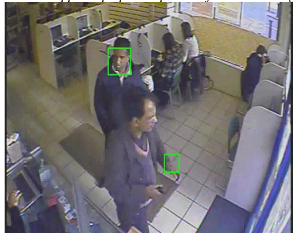
Fig.10:The same footage was passed through the OpenCV full frontal face cascade classifier considerably.
