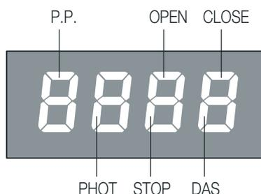
N.C. inputs are represented by the vertical segments. N.O. inputs are represented by the horizontal segments.
