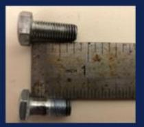
When this longer bolt is used, it presses against the starter shaft when tight and it messes up the Bendix operation.
