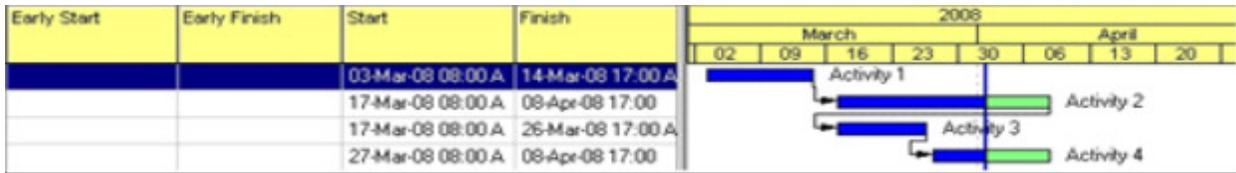
Figure 17 - Out-of-sequence Progress before CPM Calculation
