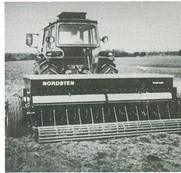
The Combi-matic drills sow both seed and fertilizer at the same time.
