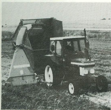
The forage harvester is mainly used for direct harvesting of grass crops.
