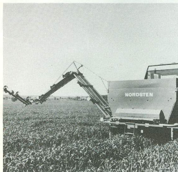
On the Air-o-matic pneumatic fertilizer distributor, the fertilizer quantity is controlled by a drive wheel and is thus independent of the driving speed.
