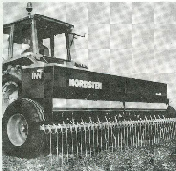
On the Lift-o-matic CLH 300 the wheels are placed within the working width and the coulters on three rows.
