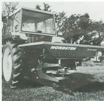
The Turbo-matic spinner can be adjusted for a constant spreading width for all kinds of fertilizer.
