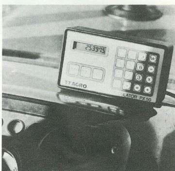
The electronic Calculator PX 50 serves as area meter, milage recorder or bale counter.
