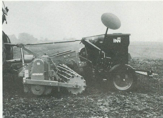
The Rotalabour in combination with seed drill for soil preparation and sowing in one process.
