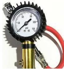
One of the gauges reads to 100 psi while the other gauge reads to 150 psi. Make sure the gauge will read to the pressure needed for your tires. There is a decal on the door jamb or "B" pillar that tells you what to inflate your tires to; it should be in every light truck and van. If it's not there or is illegible, then go to the manufacturer's website to look for the data. There is also a maximum load/pressure embedded in the tire's sidewall.
