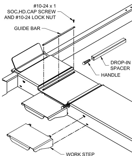
**Fig 14 – Alignment Turn Plate Installation**
