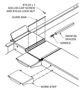
Fig 14 – Alignment Turn Plate Installation
