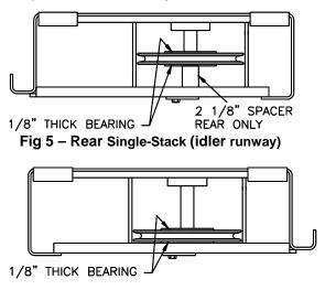
Fig 6 – Front Single-Stack (typical for idler and power runways)
