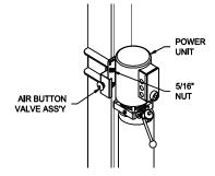
Fig 11 – Air Button & Power Unit Mounting
