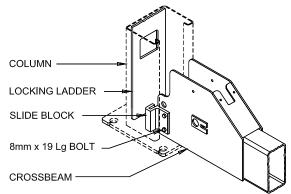
Fig 9 – Slide Block Installation
