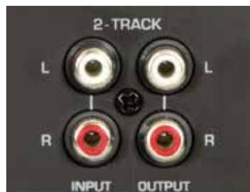
Alternatively, the line or tape output of a hi-fi amplifier with source selection switch could also be hooked up here, allowing you to easily listen to additional sources.
