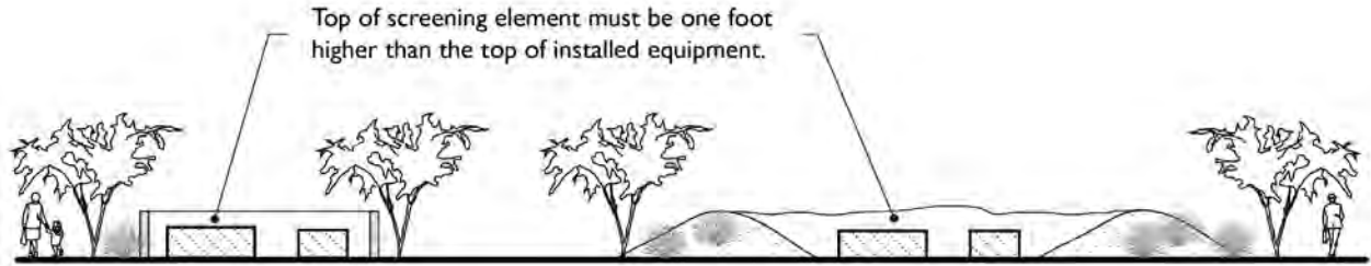
FIGURE 17.25.150(C)(2): SCREENING OF GROUND-MOUNTED EQUIPMENT
