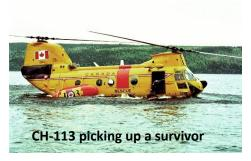
The *Labrador* had a watertight hull for marine landings and a water dam could be installed forward of the rear loading ramp for water deploying a zodiac or swimmers. An internal winch mounted in the forward cabin was used to assist pulling in cargo and was used as a backup rescue hoist via pulleys in
