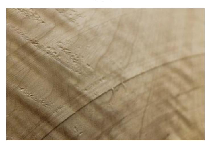
By closing the flute, the gouge will slice the wood fibers with the nose radius instead of just cutting them. Notice that the cutting edge is almost parallel to the rotation of the wood. Again, note how I rub the bevel to control the depth of cut. Slicing Cut
