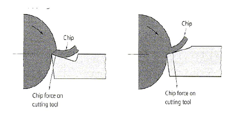
The negative rake tool actually pushes the wood fibers down and with that, the other wood fibers support the others so the fibers can be cleanly cut off.
