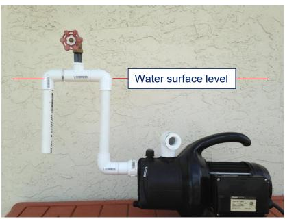
Note: When your water level is higher than the pump location, water static pressure can exceed the negative pressure resulting no suction. In that case, please set the gas inlet point higher that water surface like right picture.
