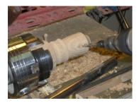
Hollow out the inside. Do not enlarge the first 1/8 to 3/16 of the bored hole. The walls should be 1/16"-1/8" thick. The hollowing should be just past the perch hole and leave about a 1/4" shoulder on the 1" bored hole. Mark the outside 1 3/4" (the bottom of the bored hole) so that when you finish turning the bottom, you won't have occasion to use four letter words like oops etc.
