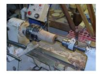
Rough turn the outside. Form the top so that it will fit in the shoulder of the 1 1/8" hole you bored in the roof. Support the turning with the tailstock.
