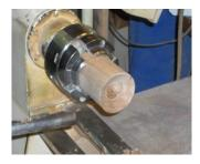
Drill a 7/32" hole 1/2" deep. This is used for a 1/4" screw chuck later.
