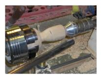
At this point you can part off the bottom or reverse turn the bottom for more elaborate detail.
