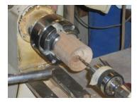
Turn the outside of the roof, support with the tailstock. Sand the roof before parting it off.
