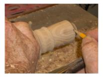
Drill the Entrance and perch holes. The Perch hole is 1/8" and the entrance hole is 1/4" to 7/32". The perch hole should be directly under the entrance hole. The holes will be positioned more accurately if they are started with a hole made by an awl or center punch.
