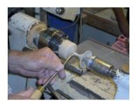
Using the 7/32" hole, mount the roof on a 1" dowel with a 1/4" lag screw in the end or on a shop built screw chuck with  $\frac{1}{4}$  20 threads for finishing.
