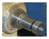
Mount the roof on the Arbor Screw Chuck. Then mount the chuck in the lathe and slide the tail stock forward to mark the center of the roof as a center punch would.
