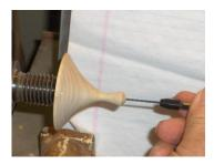
**Turning the bottom:** Start with a 1 1/2" x 1 1/2" x 3" diameter blank mounted in a chuck. Bore a 1" hole about 1 3/4" deep. *Note: The hole in the bottom should be 1/8" smaller in diameter than the hole first bored in the roof.*
