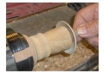
Determine the location for the perch and entrance holes. This will be the front so try to find the best grain (the "face") or the most interesting features. The perch and entrance holes should be about 1/2" apart and the perch hole should be at least 1/4" from the bottom of the 1" hole.
