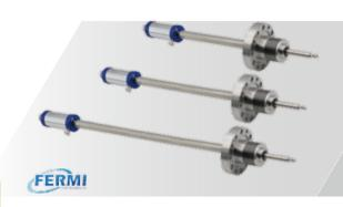
This Wobble Stick combines edge welded bellows and magnetic coupling technologies, enable the inner 8mm shaft moves linear and rotary and at the same time achieve the tilt range up to 20 degress.
