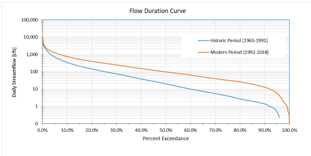
**Figure 23. Flow duration curve.** This flow duration curve is for Lac qui Parle River near Lac qui Parle River, MN (USGS# 05300000) and compares two periods, a “historic” benchmark condition (1965-1991) and the modern condition (1992-2018).
