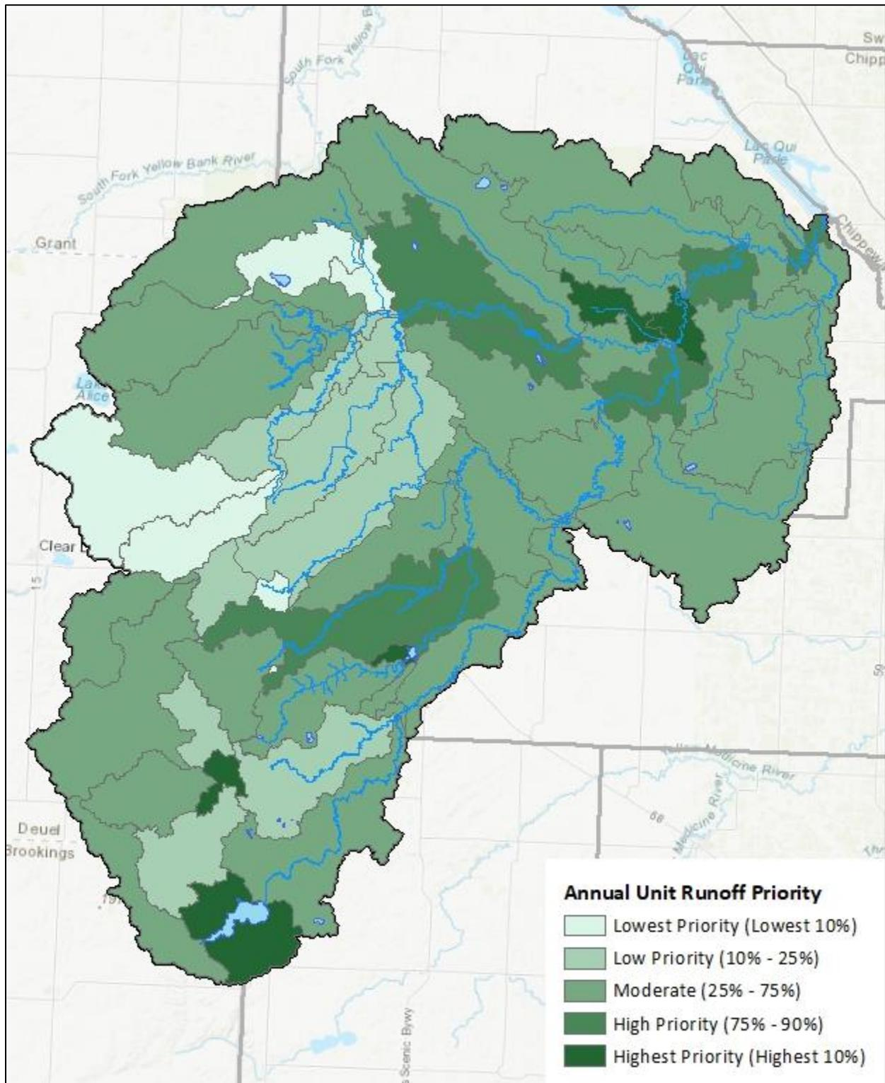
Figure 54. Subwatershed implementation priorities for the stressor altered hydrology, using average (1995-2012) annual unit runoff as modeled by HSPF.
