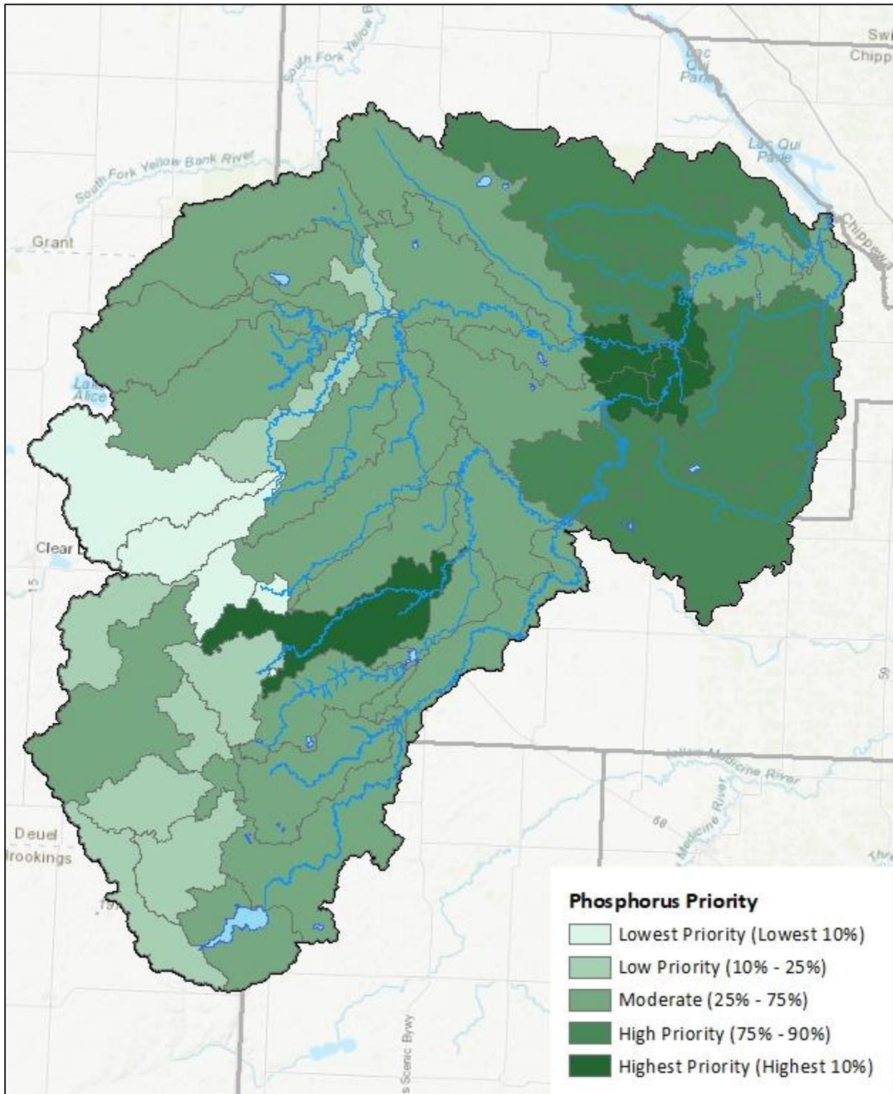
Figure 56. Subwatershed implementation priorities for the stressor excessive nutrients, using average (1995-2012) total phosphorus yields as modeled by HSPF.
