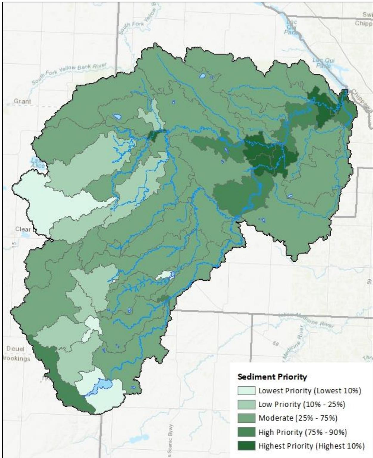
Figure 55. Subwatershed implementation priorities for the stressors elevated turbidity and loss of habitat, using average (1995-2012) total sediment yields as modeled by HSPF.
