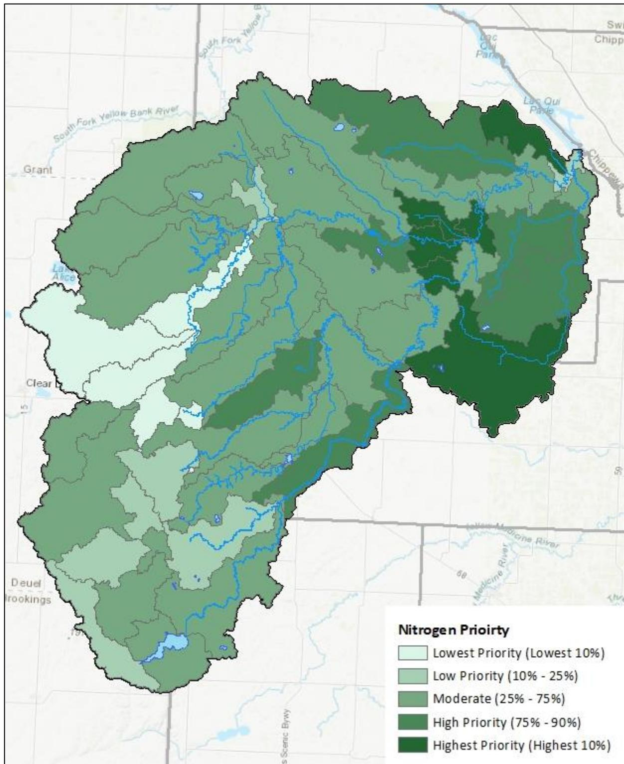
Figure 57. Subwatershed implementation priorities for the stressor excessive nutrients, using average (1995-2012) total nitrogen yields as modeled by HSPF.
