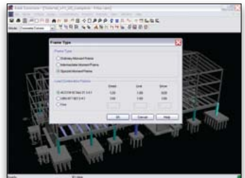
The Intermediate and Special moment frame requirements of ACI 318, Chapter 21 are implemented in RAM Concrete.
