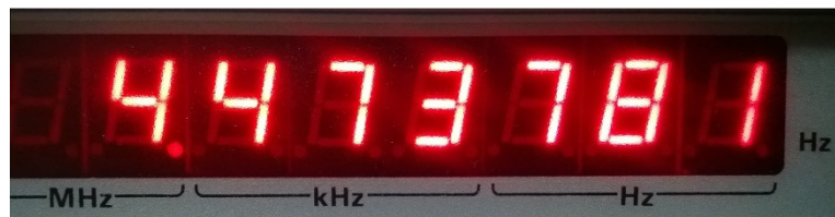
Figure 6.14 – Verifying internal VCO frequency.
