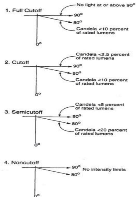
**Figure 13.** Cutoff classifications for standard outdoor or roadway luminaires
