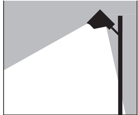
**POLE TOP-MOUNTED CUTOFF LIGHTING, SHOEBOX FIXTURE**
