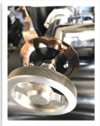
IF YOU ARE USING THE NEW 2018 BC ROASTERS WITH MANUAL DIAL DAMPER (MDDS SYSTEM) OR A PHOENIX OR SEDONA MODEL YOU CAN TEST AIRFLOW AS WELL. KEEP IN MIND THAT THE MANUAL DIAL DAMPER ACTUALLY OPENS OR CLOSES THE EXHAUST PIPE SO IF YOU ARE UPGRADING FROM AN ELECTRONIC ROASTER TO THE MDDS SYSTEM YOU WILL LIKELY NEED TO INCREASE THE SETTINGS ON YOUR AIRFLOW.
