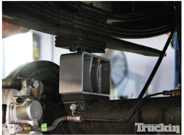
21. The rear lift is accomplished with a six-inch fabricated steel lift block that goes between the axle and leaf-spring pack.
