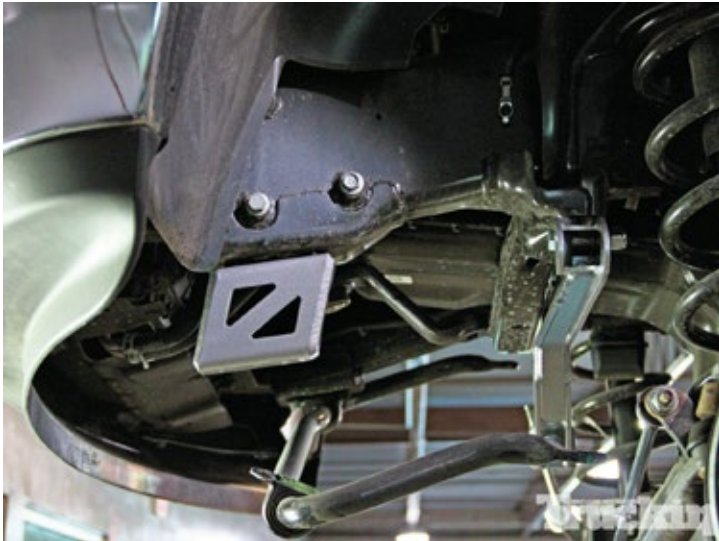
19. Since we moved the sway bar endlink mount down, we needed to move the sway bar down away from the frame. Again, the kit included a pair of sway bar relocater brackets to do just that.
