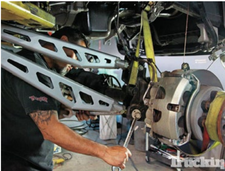
13. Finally, the long arms were bolted into the factory location on the front axle. One of the cool things about this kit is that the long arms have Johnny Joints so that they can be minutely adjusted if need be.
