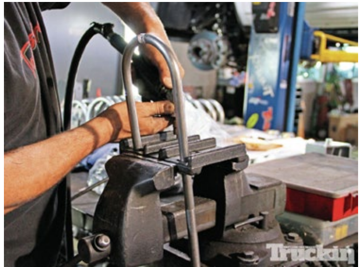
22. Rather than use the factory 9/16-inch U-bolts, McGaughys includes four 5/8-inch U-bolts. This means that the upper plate needed to be drilled out. These extra heavy-duty U-bolts will hold up to extreme towing and ensure a long life.
