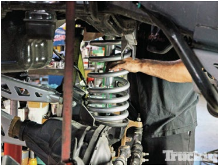
18. The next step was to install the new shock and coil spring in the factory location. McGaughys includes new shocks in their kit, but we opted to upgrade to Bilstein shocks for even better ride and handling.
