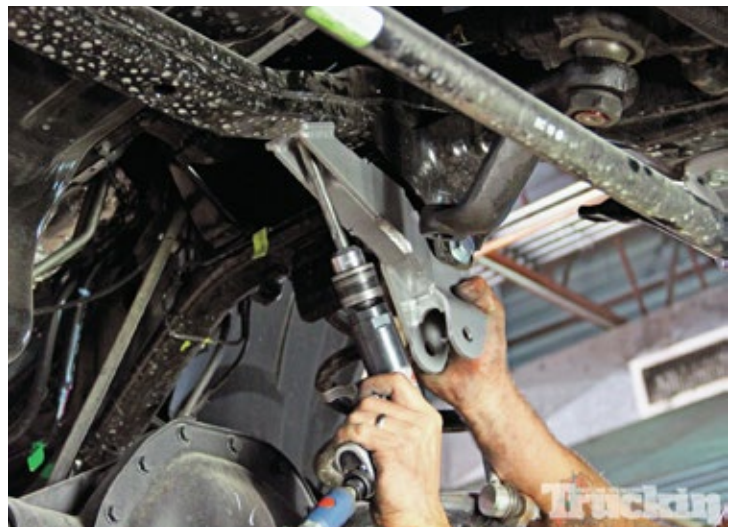
17. Another hole needed to be drilled in the frame. This one was for the track bar drop-down bracket. Once that was drilled, the bracket was bolted to the frame and was ready to receive the factory track bar.
