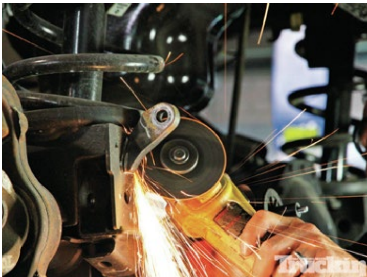
14. In order to keep the sway bar in the correct orientation, the factory mounting bracket had to be cut off. Again, we made sure to just cut the welds and not the frame.
