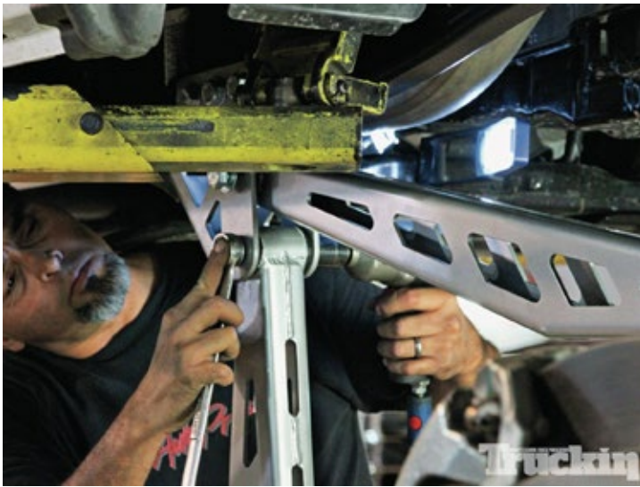
12. After the bushings were installed, the new McGaughys long arms were bolted into the new bracket that was installed earlier.
