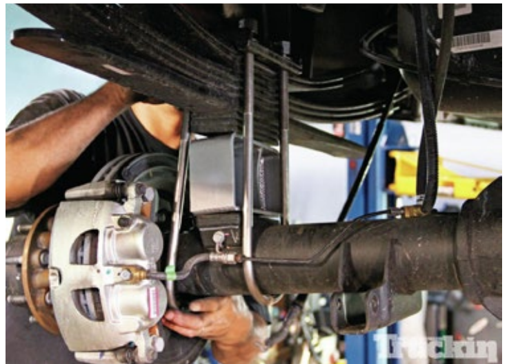
23. After the holes were drilled out, the new U-bolts and the plate were installed onto the axle and the block was sandwiched down.
