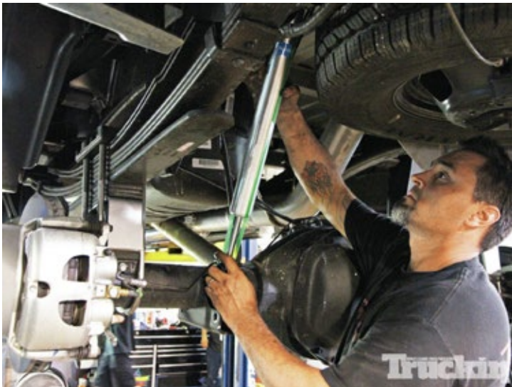
25. Finally, a new pair of rear Bilstein shocks (optional) was bolted into place and the install was complete.
