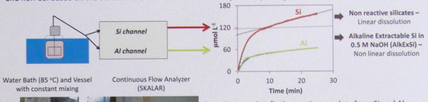
Each AlkExSi fraction is characterized also by a reactivity parameter (k) reflecting the dissolution curve "shape" and its ability to dissolve in NaOH. An average reactivity is calculated for each sample:
