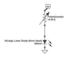
Fig. 2: A circuit diagram for the transmitter. Separate power sources were used for channel A and channel B.
