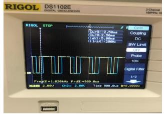
Fig 8: Waveform obtained with US Digital transmissive linear LPI 127 strip.
