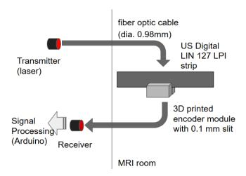
Fig. 1: A high-level diagram of the encoder, which consists of three major components: transmitter, encoder module, and receiver.
