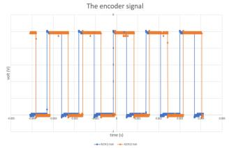
Fig 9: Voltage transition in signal A and B over time obtained by oscilloscope with US Digital transmissive linear LPI 127 strip.
