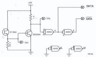
Fig. 4: A circuit diagram for the receiver, where DATA indicates the output of the encoder [7].
