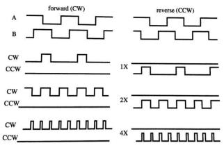
Fig. 5: Quadrature direction sensing and resolution enhancement [5].
