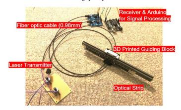
Fig. 6: Completed experimental setup of the encoder. Separate power supplies are attached to each of the laser transmitter.
