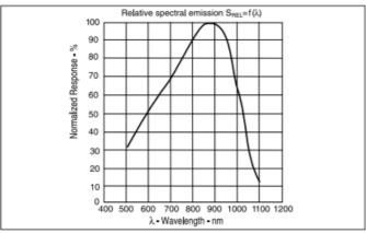
Fig 10: Typical detector response of IF-D92 versus wavelengths [6].
