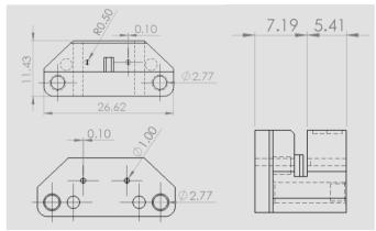
Fig. 3: A design of encoder module. Top-left: a transmitter side of the encoder module, which has a separation block between the two light source. Bottom-left: a receiver side of the encoder module. Right: the two modules are connected with the mounting hole.
