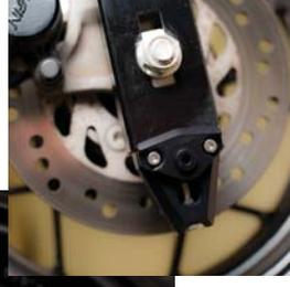
Insert photo to the left shows the correct installation of the Spool Adapter block. The installation method is the same as for the pinch blocks shown.
