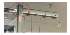
Attach the overhang to the backbone with the 2x, 4 $\ddot{o}$  long,  $\frac{1}{2}\ddot{o}$  socket head bolts and tighten them all the way using the provided  $\frac{1}{2}\ddot{o}$  nylon nuts.
