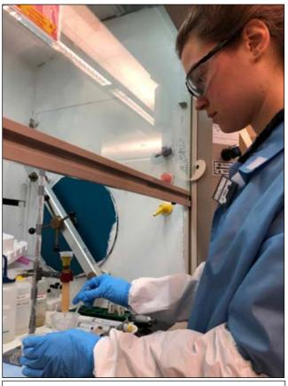
Figure 1. Sara Gilson, PhD student in chemistry and biochemistry at the University of Notre Dame, loads a neptunium-bearing solution (green) into a column for purification.
