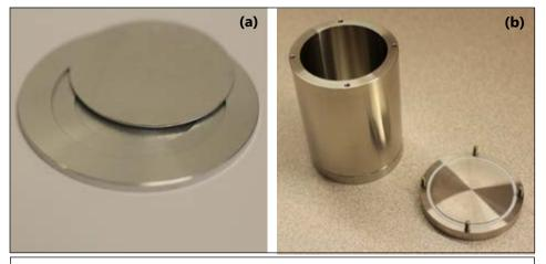
Figure 2. (a) The TOAD is used to field foils for neutron irradiation 50 cm from the NIF capsule. Foils are sealed inside the TOAD, which is removed after a shot for processing. (b) The H-TOAD container is used to similarly field several grams of material or multiple foil stacks.
