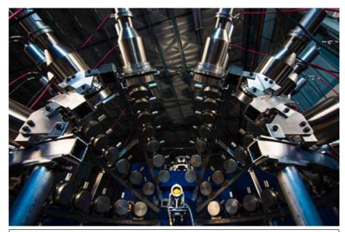
Figure 2. The Chi-Nu detector array. The Los Alamos Neutron Science Center facility produces 'white spectrum' neutrons that interact with a fissionable target (golden disc near center) and are subsequently detected by an array of liquid scintillator (shown) or lithium-glass detectors. The double time-of-flight measurement technique uses the times from the source to target to detection to infer the PFNS as a function of the incident neutron energy.
