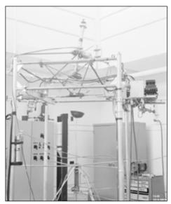
Figure 3. The Lady Godiva (high-enriched uranium) critical assembly experiment after a prompt supercritical accident involving 5 cents of excess reactivity. The National Criticality Safety Program operates the National Critical Experiments Research Center in Nevada.
