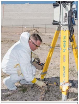
Figure 1. Expert performs soil deposition monitoring using an Ortec Detective for the purpose of quantifying and identifying trace levels of radioactivity present to advise decision makers.
