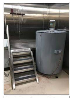
Figure 3. A large calorimeter at the University of Notre Dame is dedicated to studies of actinide chemistry and is the only such instrument in the world that can be used for measurements of transuranium compounds.
