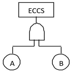
Figure3. Fault Tree of ECCS
