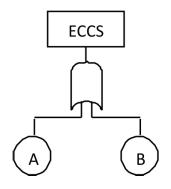
Figure6. Fault Tree of ECCS
