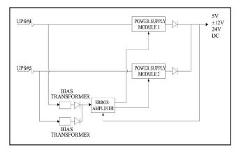
Fig.3 Current Sharing Mode Power Supply
