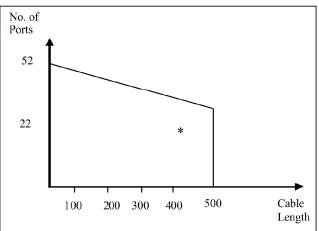
Figure: 2 Relation between no. of nodes and length of LAN cable
