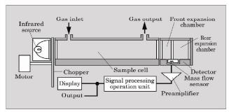
Fig.1 Configuration of single-beam type measurement unit
