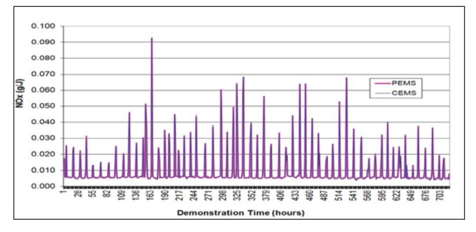
Figure 4 Time plot PEMS versus CEMS for NOx emitted by a peaking gas turbine. Comparison period 720 hours (Part 75 certification)
