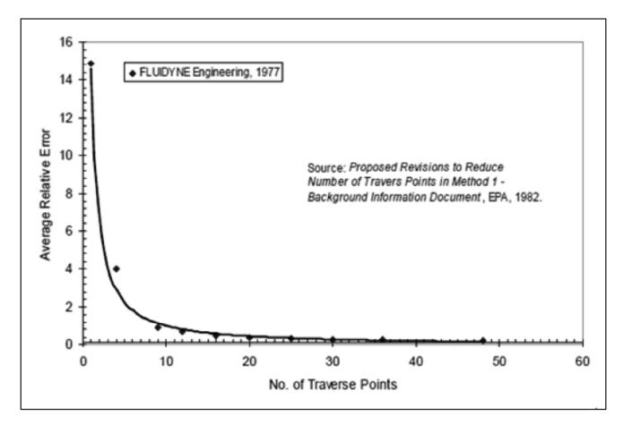
It is interesting to note that traverse point more than 20 points are required to get a relative accurate measurement of CIA/LOI.
