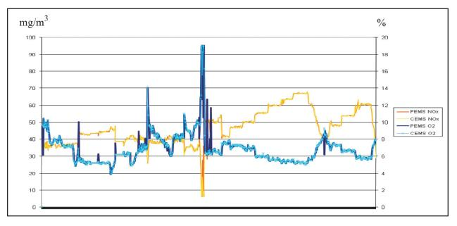
Figure 3 Comparison of PEMS / CEMS results for NOx und O2 (oil-fired boiler).
