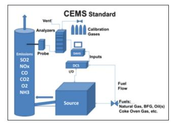
Fig. 1 Standard CEMS Configuration DAHS: Data Acquisition and Handling System
