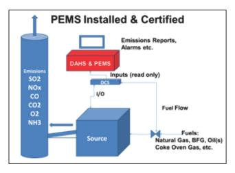
Fig. 2: Emissions Monitoring with PEMS and Data Acquisition (DAHS)
